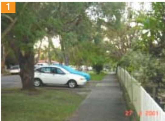
1 A partially paved footway area with a longitudinal paved strip mainly for pedestrian use.
