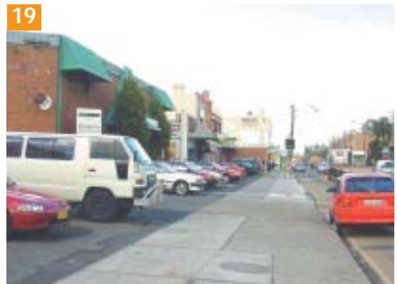
*A barrier kerb with a wide fully sealed footway.*
