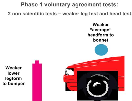
The Phase 1 tests – the only certain pedestrian sub-system tests in the agreement - have been roundly criticised by experts as non-scientific (Janssen 2001, Hobbs 2001, Lawrence 2001). The Phase 2 tests mention the possibility of adopting EEVC by 2010 but 'equivalent measures' are allowed and, as previously noted, the second Phase would be subject to a review in 2004.
